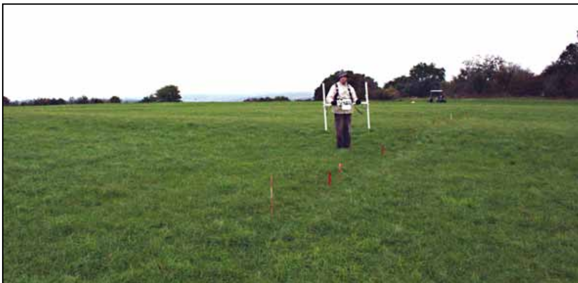
Figure 2.1 The Bartington magnetometer in use at the site on Bathampton Down.
