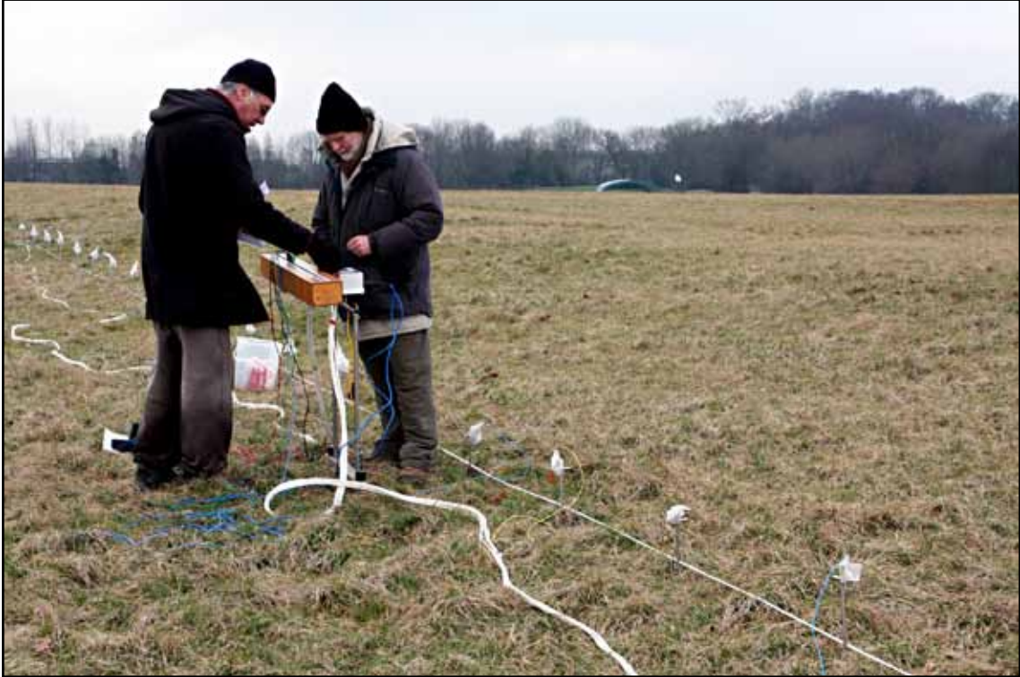
Figure 2.3 Resistivity profiling on the site.
