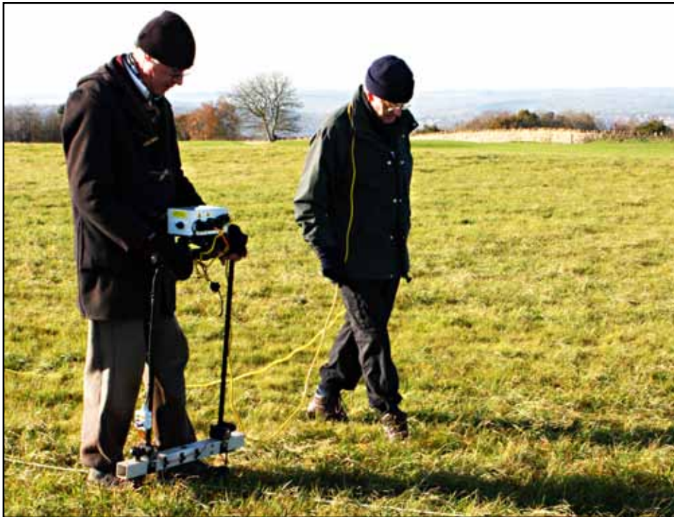
Figure 2.2 Twin probe resistance meter on the Down. The background view is to the west.
