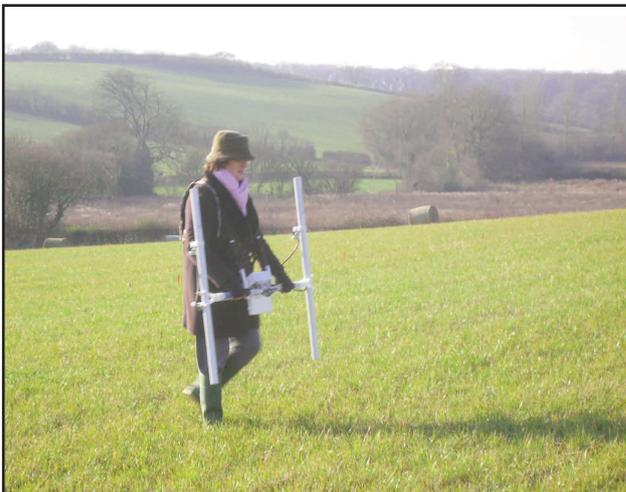
Bartington over the main part of a field while using the FM around the edge.
