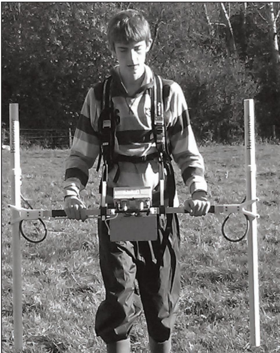
The following day the two grids of interest were surveyed with the resistivity meter and the results revealed an area of high resistance, looking suspiciously structure-like and adjacent areas of low resistance, matching the magnetometer survey (*see Figure 3*). This area of interest will hopefully be explored by excavation later in the project.
