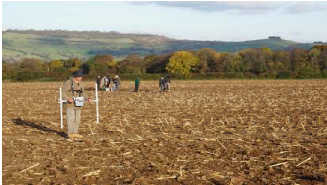
Figure 2.1. Bartington 601-2 magnetometer in use during the survey. Resistance survey in progress in the background. This was in the first week, before the field was rolled.
