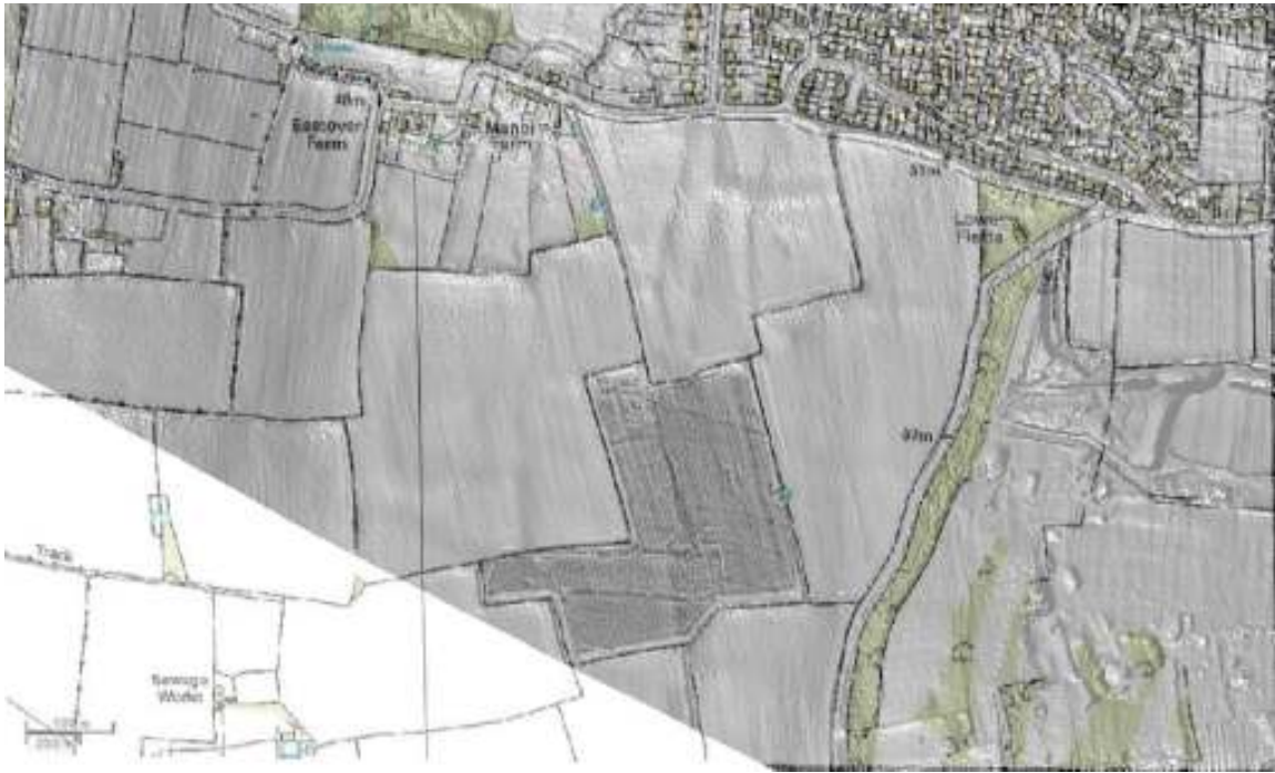
Figure 4.3. Magnetometry of Coffin Field, showing surveyed features and their relationship to features observed by lidar.
