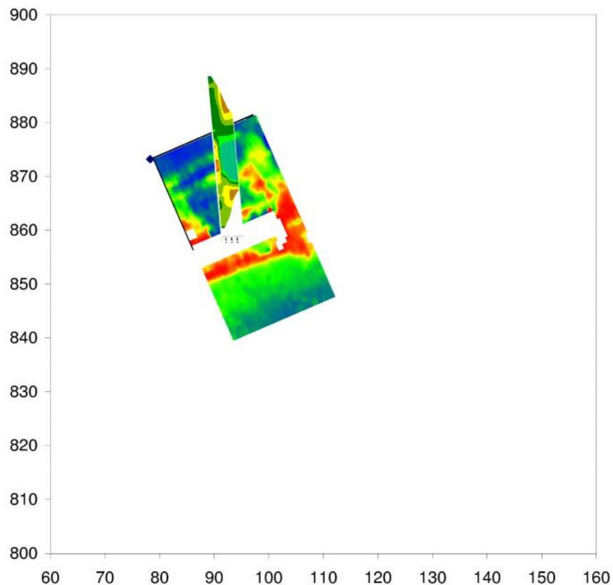
**Figure 3.9. Streamside resistance plot shown with profile position overlaid. Note that the plot has been overlaid on Ordnance Survey coordinates, so, for instance, point 100, 850 should be read as ST 69100, 63850, or 369100, 163850.**
