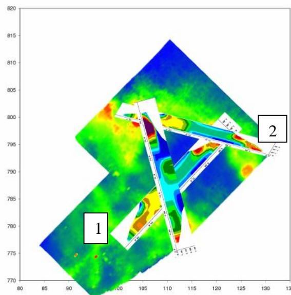
Figure 3.4 Profiles shown overlaid on resistance plot.
