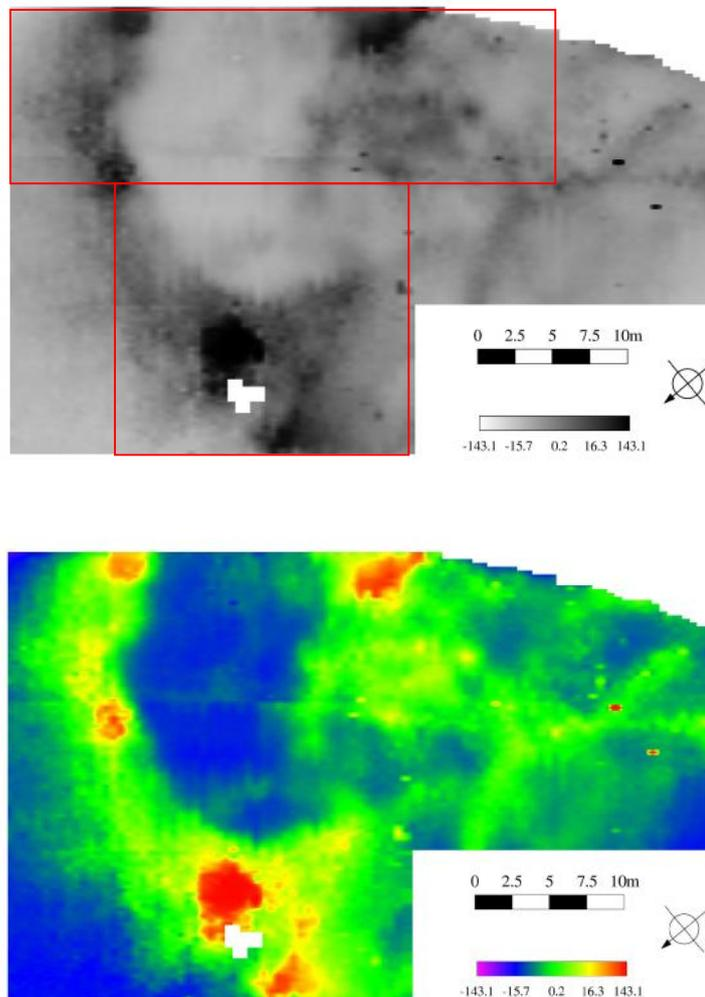
Figure 3.1. Twin probe resistance on the mound. Greyscale and colour plots. The red outline on the greyscale plot indicates the area shown in figure 3.2.
