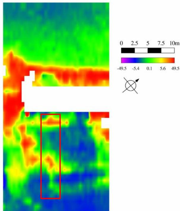
**Figure 4.2. Resistance plot streamside, with red box indicating area of most profitable excavation**
